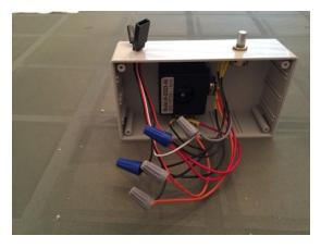
Take the remaining servo extension wire that has all three wires, and feed it thru the hole. Then attach the black wire to one of the pots on the joystick (middle wire). Attach the red wire to the other pot on the joystick (middle wire). Attach the white wire to the middle wire on the potentiometer.
