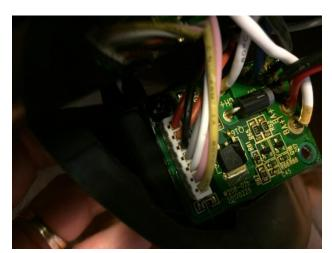
On the underside, you will find another circuit board. Remove the screws holding this to the cover. Remove the bundle of wires attached to the long white connector by unclipping the connector.
