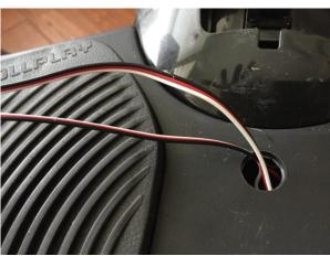
Then drill a hole thru the foot board for the servo extension wires. Connect them with another set of servo connection wires and feed thru the hole. The replace the foot board.
