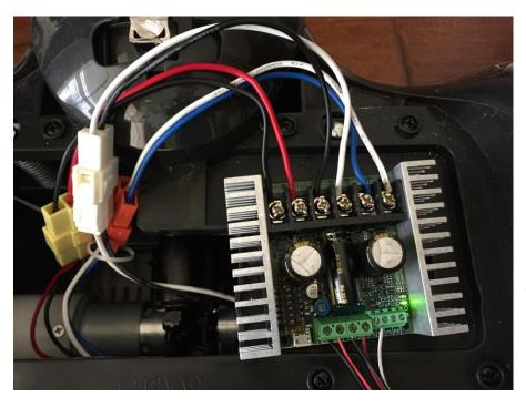
Take your two remaining servo extension wires. On the set that does not have a white wire, wire the black wire to 0V and red wire to 5V. With the remaining extension wire, wire the black wire to S1, the red wire to S2, and the white wire to A2. Attach the servo wires to their mates on the joystick control box, and the power/motor connectors to their color matches mates. It should look like the next picture:
