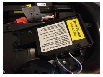
Unscrew the box holding the electronics. You will need to remove the screws holding the top cover to the base first, and then remove the top.
