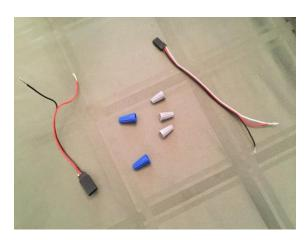
Take the female end of the servo extension wire (the one missing the white wire) and the male end of the other extension wire. You will now need 2 medium sized wire nuts and 2 small wire nuts.
