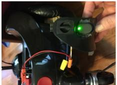
Check you wiring by plugging the connector back into the battery. If this works, then you can disconnect it, and feed the connector back thru the device like it was before.
