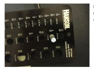
Figure out what size hole you will need to drill in your control box for the potentiometer. Here it would need a 9/32 hole to pass easily thru the hole to be mounted.
