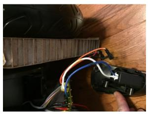
Once you have removed the switch, disconnect the 3 wires attached to the switch. The only 2 wires still attached to the cover should be the blue and white wires which go to the charging port. Clip and strip the end of the white wire where it attached to the circuit board.
