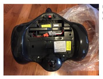
Remove Uprider from packaging. Remove the footboard. Disconnect the orange plug from the battery.
