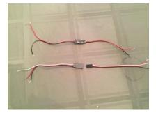
Take 2 servo extension wires (I prefer the 60 cm ones). Cut them in half, and then strip the ends. On one set of wires, cut the white wire at the connector.
