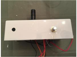
Take the joystick and feed thru the 1" hole. Then attach to the box with the mounting rings and screws that came with the joystick. On the side, feed the pot thru one of the holes, and attach the mounting washer and nut.
