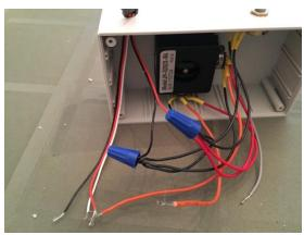
Feed the servo connector that only has a red and black wire thru the remaining hole. Use the 2 medium wire nuts to attach the positive wires (all on far left of the 3 pots) to the red wire and the negative wires (all on the far right of the 3 pots) to the black wire.
