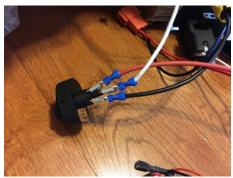
Once the glue is cool and the on/off switch is secure, take the 3 wires with wire connectors and attach: red to supply, black to earth, and white to load. (This picture shows the wiring- but do this AFTER you mount the switch to the cover)
