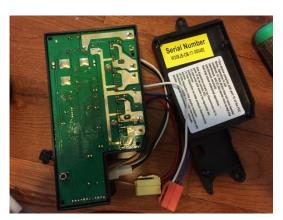
Find the motor controller that originally came with the Uprider. Clip the 3 big wires where they attach to the motor controller. Strip 1/8" of the end of each wire.
