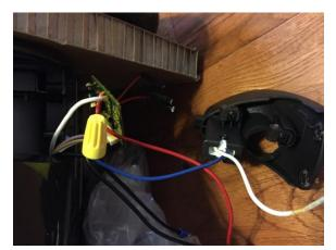
Next, get the single piece of black wire that you added the connector to, and with a large wire nut, attach the 3 black wires and one blue wire.
