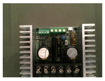
This is your sabertooth 2x32 motor controller. Pull it out of the box and loosen all the screws which take a Phillips head screw driver.
