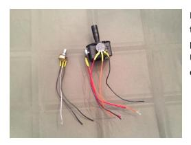
For the joystick and speed control, solder 18-22 gauge wires to the 3 pots (2 on the joystick and one on a potentiometer). I like using unused wire salvaged from the Uprider. Cover connections with heat shrink and strip the ends 1/4 ".
