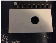
Drill two 9/32" holes in the side of a project box. (one hole will be for the pot, and one will be for your wires.) Drill a 1" hole in the base of the project box. (this is for your joystick)
