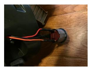
Use a spade screwdriver to push the on/off switch out of the cover, by pushing from the inside of the cover on the clips of the on/off switch. It should come out of the front of the cover.
