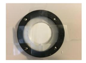
Take the mounting ring for the joystick and tape it to the top of the project box, centered on the 1" hole. Then drill the 4 holes of the mounting ring thru the box.
