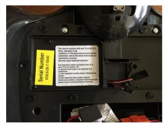
Screw the top on the enclosure. Connect the orange, yellow, and white connectors to their mates, and then replace the holder in the Uprider. Remember to screw it in.
