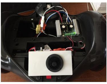
Once everything is hooked up, turn on the power and the green light should turn on with the sabertooth. The joystick should respond appropriately for right and left; forward is pulling the joystick down, and reverse is pushing the joystick forward. The overall speed is controlled by the potentiometer on the side.
