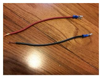
Take 2 pieces of 16 gauge stranded wire, about 6-8" long. Strip the ends, and then connect a wire connector to one end .
