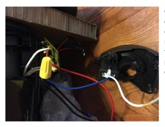
Clip the remaining red wire that is attached to the circuit board (this goes to the battery). Strip the end. With a wire nut, attach the extra piece of red wire you cut, the red wire you just cut from the battery, and the white wire from the charging port. If done correctly, you now have no wires connected to the circuit board by the cover.
