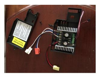
Once you have verified that your wiring works, you can either mount your motor controller outside of the Uprider, or inside the Uprider, where the previous controller was. For this, we will put it in the enclosure where the previous controller was. The wires/connectors to the battery and motor are fed thru the side, and the wires to the joystick control box will be fed thru the lid.
