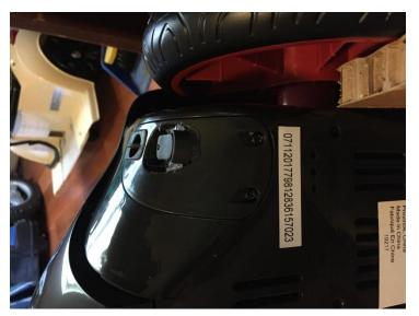
Replace the back cover using the 2 screws.
