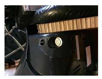
Next, locate the on/off switch and charging port. Remove the 2 screws just below the on/off switch, and gently pull forward to reveal the wiring inside.
