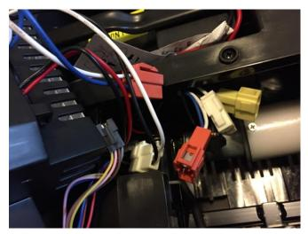
Underneath the box, you find 3 connectors (yellow, white and orange). Disconnect these. Also disconnect the little black connectors so you can remove the electronics box completely. It should look like this once it is removed:
