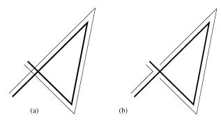
Fig. 4. Comparison between (a) the untrimmed offset curve and (b) the offset curves after clipping.
