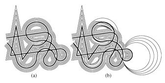
Fig. 22. The thick original polyline curve is an open curve. The thin offset curves on both sides of the original curve are from (a) our offset algorithm and (b) AutoCAD 2004 with the offset distances 15, 25, 35 and 45 mm, respectively.
