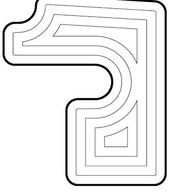
Fig. 27. Offset results with the distances 5, 10, 15, and 20 mm.
