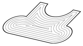
Fig. 24. Offset results with the distances 5, 10, 15, 20, 25, 30, and 35 mm.
