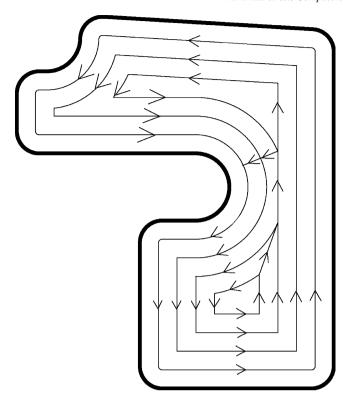
Fig. 28. Tool paths for pocket machining.
