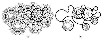
Fig. 23. The original polyline curve is closed and contains small arcs. The thin offset curves on both sides of the original curve are from (a) our offset algorithm and (b) AutoCAD 2004 with the offset distances 15, 25, 35 and 45 mm, respectively.
