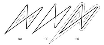
Fig. 1. The offset results from (a) AutoCAD2004, (b) AutoCAD2002, and (c) the algorithm in this paper.
