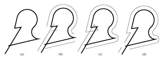
Fig. 19. The offset curves are obtained step by step: (a) the original polyline which comprises four line segments and two arcs; (b) the offset curves of all the segments of the original curve; (c) the untrimmed offset curve is obtained by Algorithms 1–4; (d) the final offset results after applying the clipping algorithm.
