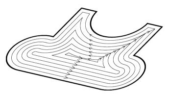
Fig. 25. Tool paths for pocket machining.
