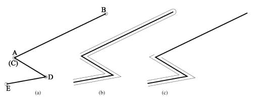
Fig. 20. The comparison between the offset results of an overlapping polyline curve: (a) the original curve with two overlapping line segments AB and BC; (b) the offset results from our offset algorithm; (c) the offset results from AutoCAD 2004.
