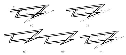
Fig. 12. The procedure of the clip algorithm: (a) two untrimmed offset curves are obtained after Step 1a; (b) the offset result after Step 1 (dual clipping); (c) one general closest point is obtained; (d) the offset result after Step 2 (general closest point pair clipping); (e) the offset results on both sides of the polyline.
