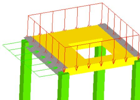
Each load case has its unique number, in the example below self-weight load - 1, live load – 2, wind load – 3.
