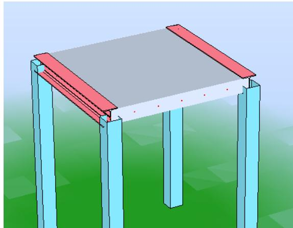
Preparing the list of points defining the slab contour; in the example below the contour coordinates are equal to the coordinates of previously defined nodes, program will automatically connect the slab contour with appropriate nodes in course of structural mesh generation.
