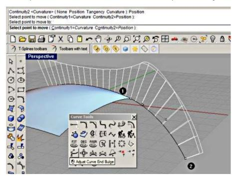
Once we are satisfied with this curve, we can proceed to create the other curve to match the other surface edge. Use the same method as described to ensure curve is curvature-matched to the edge as well. See illustration below of the other curve.
