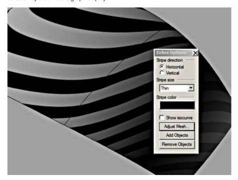
What we have illustrated here is just a simple example. If we have additional adjacent surface edges to match to, the surface from network of curve tool can provide surface continuity matching options for all sides of its boundaries.
