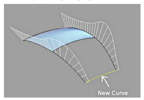
Next, using **Surface from Network of curve**, create the surface. Remember to set the **Edge matching**option to **Curvature** at the Options dialog. In this case, this is indicated as edge D. This is very important as surfaces **do not automatically** become curvature-matched even though the curves used to create them are.
