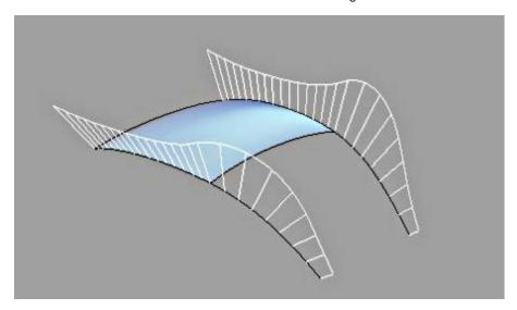
Now, we can use a surface tool with continuity to create the surface. In this case here, a new curve is created as shown below. The control point is turned on to adjust the profile to give it a slight bulge.
