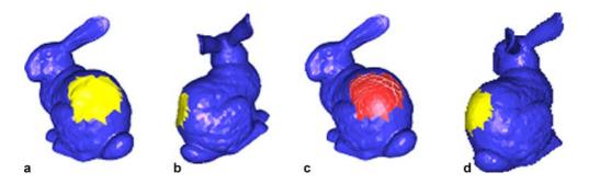
Fig. 7a–d. Reconstruction of the patch mesh. a The initial patch mesh (*yellow*). b The reconstructed mesh based on the harmonic equation. c The torn patch mesh after performing triangles rotation (*red*). d The reconstructed mesh based on the Poisson equation
