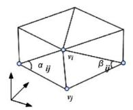
Fig. 5. Angles for the Poisson equation
