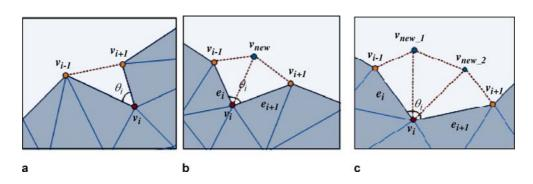
**Fig. 3a–c.** Rules for creating triangles: **a**  $\theta_i \leq 75^\circ$ ; **b**  $75^\circ < \theta_i \leq 135^\circ$ ; **c**  $\theta_i > 135^\circ$
