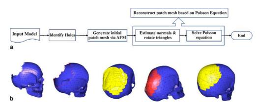
Fig. 2a,b. Algorithm flowchart and its illustration. a The flowchart. b The illustration of flowchart
