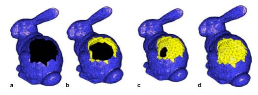
Fig. 4a-d. Process of AFM. a The original hole; b and c two intermediate stages; d the initial patch mesh created
