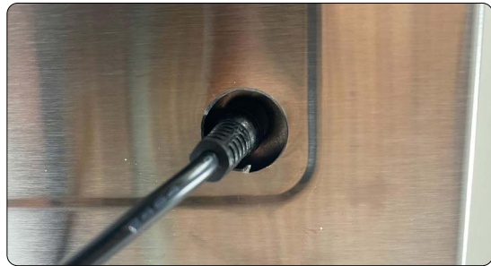
Figure 4. Holes with barrel jack connector threaded through.
