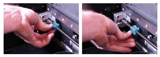
Rotate the top of the thread cleaning tool toward the front of the printer. The thread cleaning tool moves along the X-axis lead screw toward the right of the printer.
