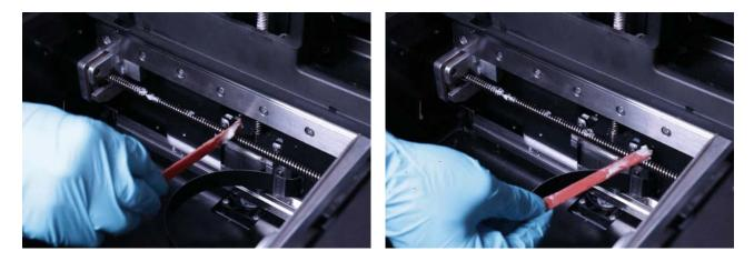
Apply small amounts of the new grease along the length of the X-axis lead screw. To watch a short video demonstration, click <u>here</u>.
