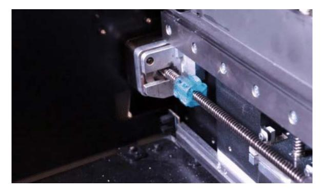
STEP 3: ROTATE THE LEAD SCREW THREAD CLEANING TOOL
