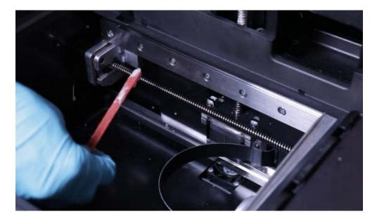
Place a small amount of lithium-based grease (approximately two pea-sized drops in total) on an applicator, such as a tongue depressor or coffee stirrer.
