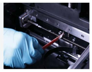
Over time, the anti-backlash nut on the X-axis lead screw can degrade and leave a black residue in the grease on the lead screw. This debris can cause the Light Processing Unit (LPU) housing to stall or generate noise during printing.
