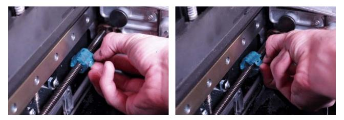
Unclip the lead screw thread cleaning tool. Remove the tool from the printer cavity. To watch a short video demonstration, click <u>here</u>.
