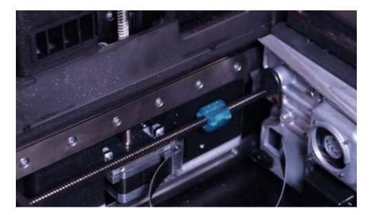
Continue rotating the thread cleaning tool until it reaches the LPU housing at the right end of the X-axis lead screw. To watch a short video demonstration, click <u>here</u>.
