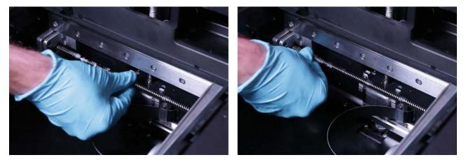
Using your gloved fingers, spread the grease along the X-axis lead screw. To watch a short video demonstration, click here.
